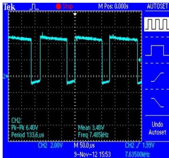
**Fig 3.2: Gate pulse at 1000gm for 1400rpm**
