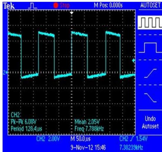
**Fig 3.1: Gate pulse at 1000gm for 1350rpm**
