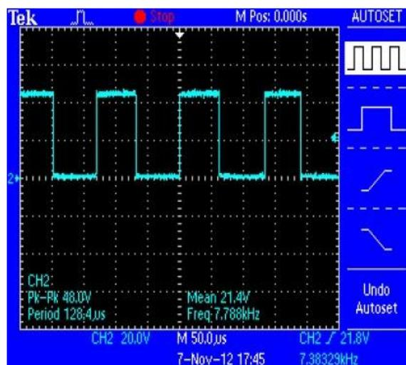
**Fig 3.3: Gate pulse at 1000gm for 1440rpm**
